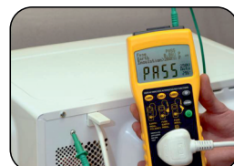
ELECTRICAL APPLIANCE TESTING
